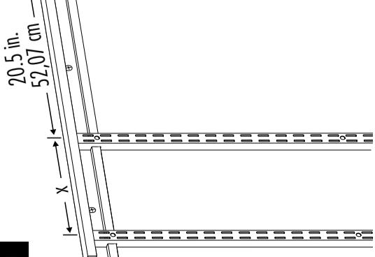
**IMPORTANT:** This product is designed to be installed onto hang standards (not included) which are part of the ClosetMaid® ShelfTrack™ system. If hang standards have been previously installed, it will be necessary to re-position hang standards as indicated and re-secure to wall.
