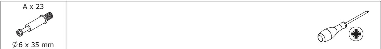
Screw eccentric rod(A) into board 9 at first. Flip to back, screw eccentric rod(A) into as well.
