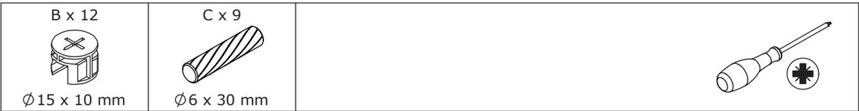
Attach board 9 to board 12, 11, 14 and 15 using wooden dowel(C), add cam lock(B) into and turn clockwise to tighten as shown.
