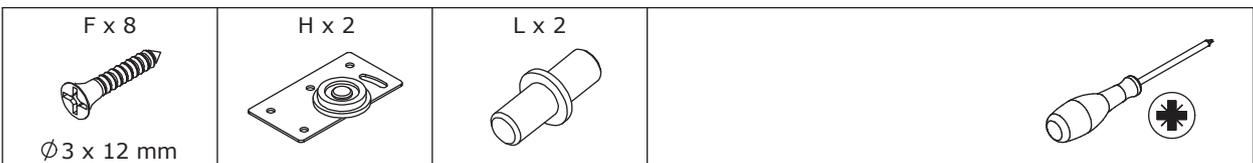
Fix part(H) to board 17 using screw(F) as shown. Insert part(L) into bottom.
