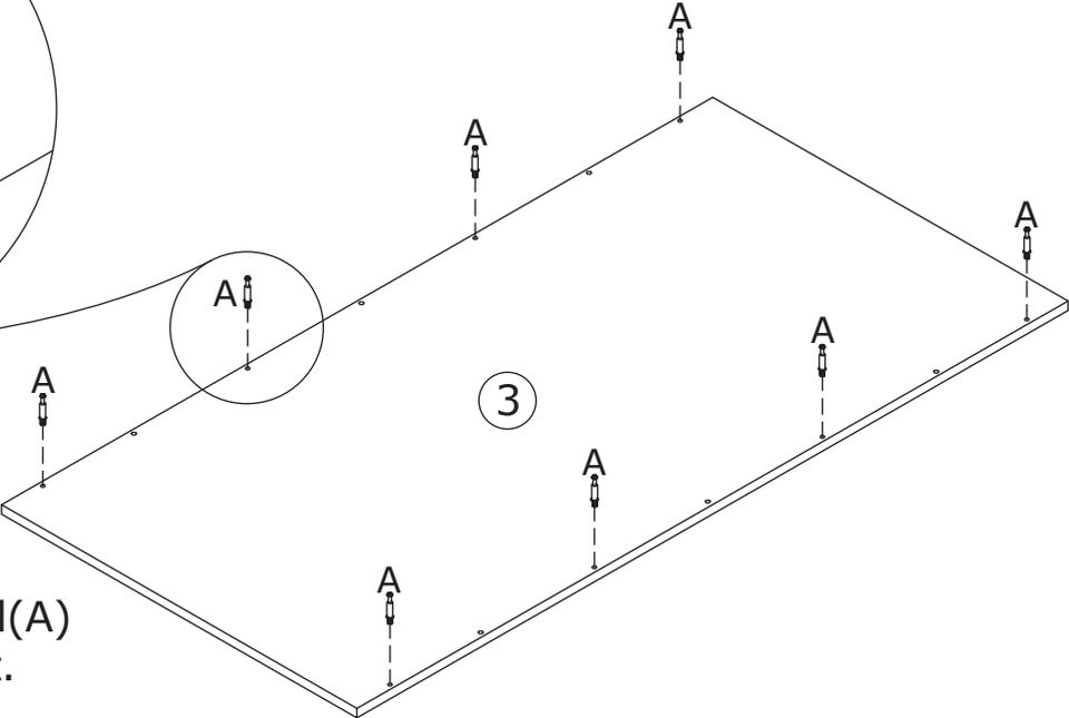
Screw eccentric rod(A) into board 3 at first.
