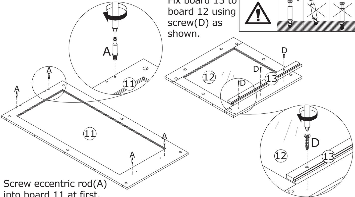
Screw eccentric rod(A) into board 11 at first.
