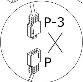
The arrows on the interface must be aligned before connecting.
