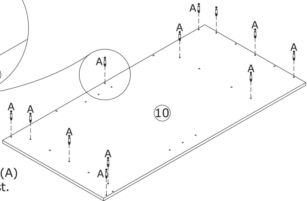
Screw eccentric rod(A) into board 10 at first.
