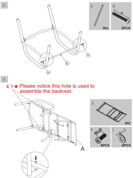
4.2 ★ Please assemble this screw first, so that the next 3 screws will be very easy to tighten.
