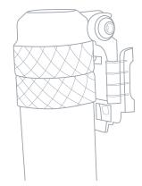
3. Locate the Valve and Tube Assembly. Connect the tube end of this assembly to the left insert on the left Filter Adapter.
