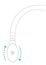
2. Disconnect the current cold water supply line under your sink.
