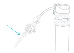
6. Remove the plug from the water inlet (#18) located on the back of the unit. To do this press on the push connect ring in towards the cooler and remove the plug at the same time. 7. Locate the second Small PE Tubing. Connect one end of the Small PE Tubing to the right side inlet of the right Filter Adapter. Connect the other end of that Small PE Tubing to the water inlet (#18).
