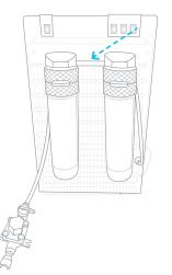
4. Connect the PE Tubing (20'), that is connected to the water source, to the open end of the Valve and Tube Assembly. Make sure that the valve is in the off position (perpendicular to the PE Tubing).
