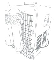
8. Locate the valve on the Vale and Tube Assembly. Turn this valve to the on position (parallel to the PE Tubing) to allow water to flow through.
