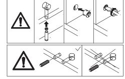
Insert back board 14 along available grooves as shown. Attach board 13 to board 11 and 12 using wooden dowel(E), add cam lock(F) into board 11,12 and turn clockwise to tighten as shown.
