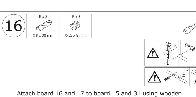
Attach board 16 and 17 to board 15 and 31 using wooden dowel(E), add cam lock(F) into board 15,31 and turn clockwise to tighten as shown.
