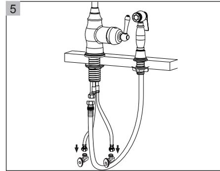
Connect the hot and cold water supply lines of the faucet to the water supply valves.
