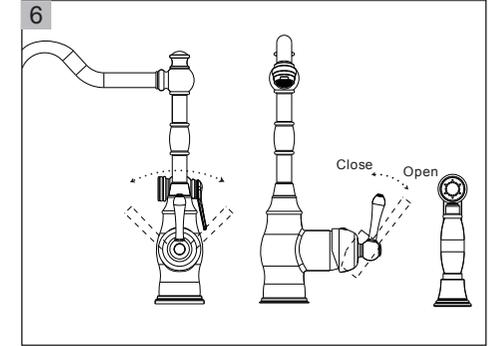
Open the valve, then turn the handle according to the sign of C and H on the handle to regulate the temperature of the water. (C=Cold,H=Hot)
