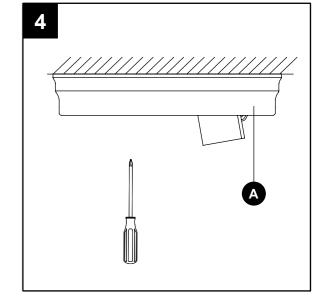
Install light bulb (not included). Use one 60-watt max. standard-base bulb or one 13-watt standardbase CFL bulb.
