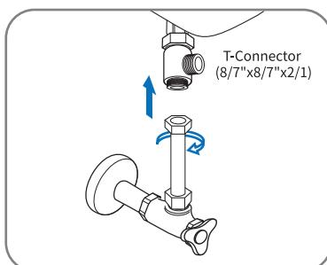
Connect the T-Connector to the water tank supply inlet.
