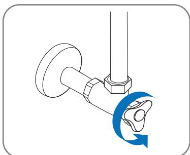
※ Please check on each connection that make sure there are no water leakage.
