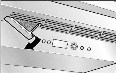
2. Remove the used Odor Filter and replace with a new Odor Filter.
