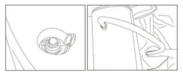
• Step d. Switch on the power and activate the BUBBLE button to begin the self-inflation process. During this time, assist the hot tub in unfolding. When the pool is properly inflated, press the BUBBLE button again to stop inflating.
