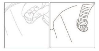
• Step c. The cover on the air valve on the outer wall of the spa should be unscrewed and the inflation hose inserted directly into it.
