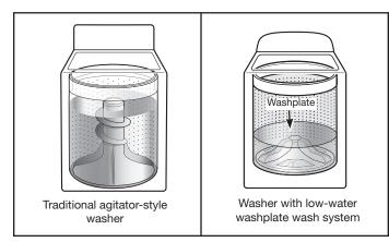
The most striking difference in your new washer is the low-water washplate wash system. The washer automatically adjusts the water level to the load size—no water level selector is needed.
