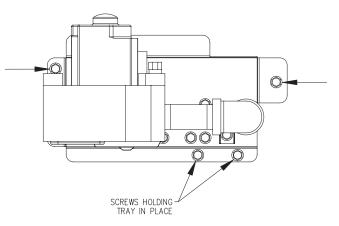
Fig. 27: Gas Valve Removal
