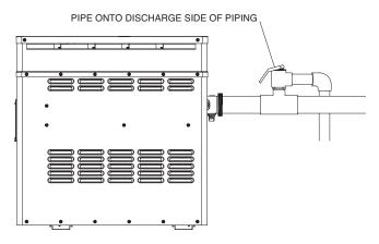
Fig. 14: Pressure Relief Valve Installed
