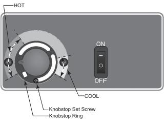
Fig. 17: Water Temperature Thermostat
