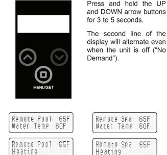
NOTE: When in remote operation, the keypad mode and temp buttons are disabled.
