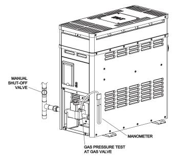
Fig. 9: Location of Gas Pressure Adjustment
