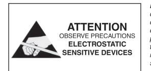
**Note:** Electrostatic Discharge (ESD) damage can be caused by direct or indirect contact with the wiring or circuit board. When one walks to the heater area, an electrostatic charge accumulates on the body. Contact of a finger allows the body to discharge, possibly causing device damage. This damage can be limited if the service person discharges himself, following ESD preventive/ removal practices, and holds on to the heater enclosure for 5 seconds before proceeding.
