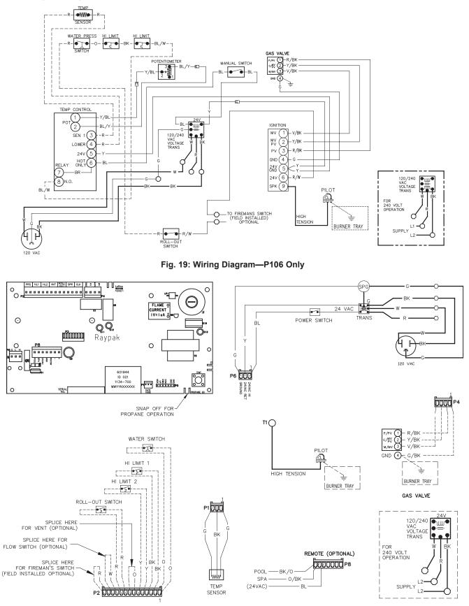
Fig. 20: Wiring Diagram—P156 Only
