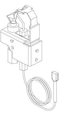
Fig. 28: Spark to Hood Pilot
