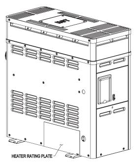
Fig. 2: Location of Heater Rating Plate
