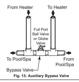
**NOTE:** Do not use a gate valve as an auxiliary bypass valve.
