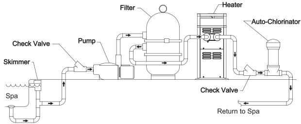
Fig. 1: Spa/Chlorinator Setup
