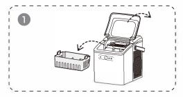
Clean it by a soft cloth with warm water and vinegar. Clean the water filter, ice shovel and the evaporator to avoid dirt buildup.
