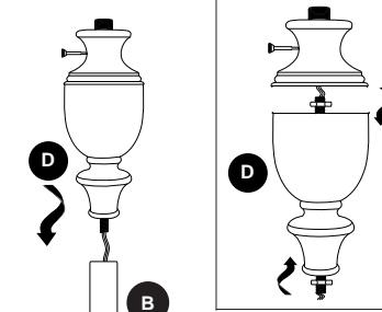
When D is **too loose**, tighten nuts securely at top and bottom of D.
