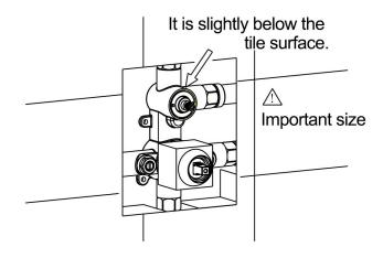
4. The water outlet of the hand shower is slightly lower than the tile surface.
