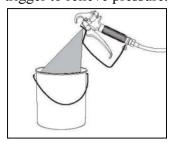
4. Turn trigger lock knob to locking position.
