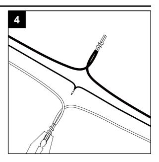
5. Attach wire nuts (CC). Tape wire nuts (CC) and wires together.
