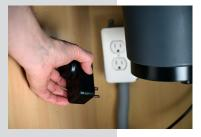
Step 4 Remove single outlet power module from power receptacle.
