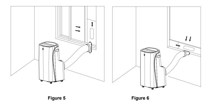
**Important Notice:** The length of the exhaust hose shall be 11-59 inches, and this length is based on the specifications of the air conditioner. Do not use extension tubes or replace it with other different hoses, or this may cause a malfunction. Exhaust must be unobstructed; otherwise it may cause overheating.
