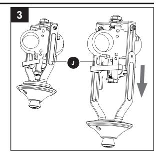
4. Once maintenance has been performed, simply lift the glass bowl (N) up to its original position. The light kit fitter (J) is secure once it clicks into place.
