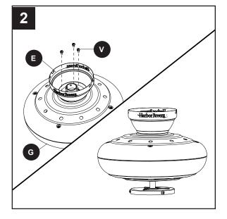
Raise the fan and place the canopy (E) on the hook on the mounting bracket (D), temporarily leaving hands free for the wiring process.
