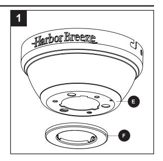
Remove three Phillips-head closemount screws (V) from the top of the motor assembly (G). Align the canopy (E) with the holes in the top of the motor assembly (G), then re-install the Phillips-head closemount screws (V) to secure the canopy (E) to the top of the motor assembly (G).
