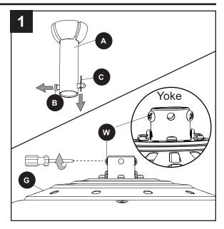
Insert the downrod (A) through the canopy (E) and yoke cover (O). Feed the wires from the motor assembly (G) through the downrod (A).
