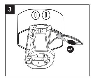
Note: Closemount installation will not use the downrod (A), yoke cover (O) or canopy cover (F).
