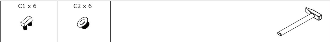
Knock part(C1,C2) slightly into the holes in panel 2&3 as shown.
