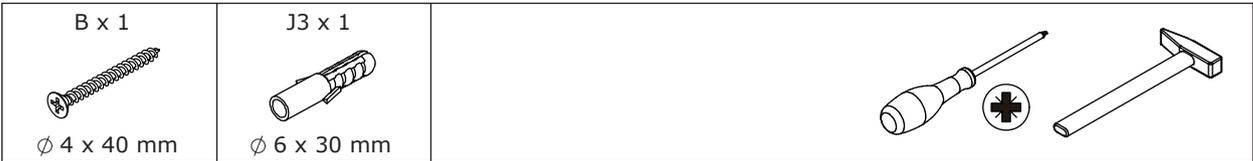
Install anti-tipping device with part(J3) and screw(B) as shown.
