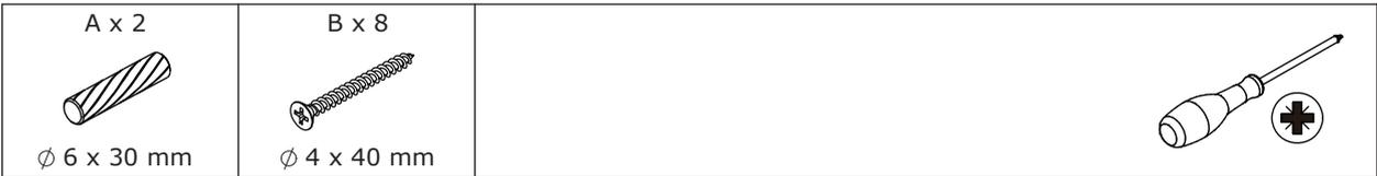
Attach panel 2 to assembled part in step 4, using screw(B) and wooden dowel(A) as shown.
