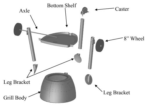
**Step 2**Attach BOTTOM SHELF to LEGS with five 1/2 inch hex bolts and lock washers.
