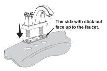
2. To tighten the mounting nuts.
