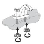
3. Connect and tighten the hot & cold supply hoses.
