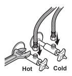
4. Turn on the water supplies. Check all connections for leaks.
