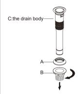
**2** Slide the drain body C through the hole in the sink.
