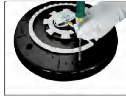
Step 4. Remove the main engine chassis screws.
