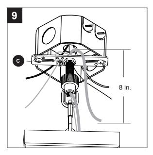
10. Separate the two fixture wires all the way to the mounting bracket (C). Strip 1/2 in. of insulation from the end of the wires. Twist the stripped ends of each strand of wire within the insulation with pliers (not included).
