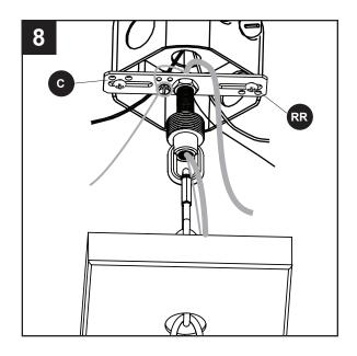
9. Depending on the length of chain (I) you use, you may need to cut the lead wires back to simplify the wiring. Take the lead wires and make sure that you have pulled them all the way through the top of the mounting bracket (C) and measure 8 in. of lead wire, and then cut the excess wire off with wire cutters (not included).
