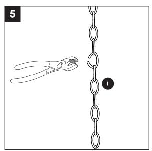
6. Unscrew the nut on open link (H), connect the chain (I) to the decorative ring (B), then close the open link (H). Weave the wires from the fixture (A) through the loops of the chain (I).
