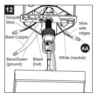
13. Wrap electrical tape (not included) around each individual wire connector (AA) down to the wire.
