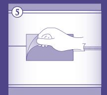
Peel the protective backing from the tape.
