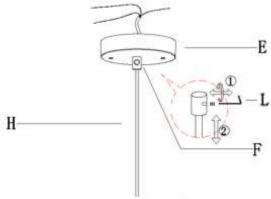
6. If needed, cut off the extra power cord length on the fixture 2 wires cord and green ground wire so that they all are at least 6 inches (152.4 mm) long within the outlet box
