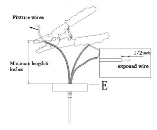
7. Carefully pass wires through the mounting plate assembly (A) Secure the mounting plate assembly (A) to outlet box with the outlet box screws (D).
