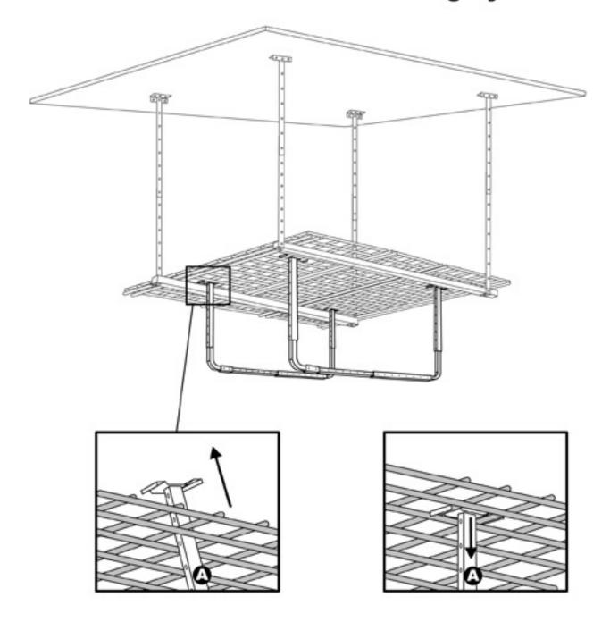
Determine location needed for storage & insert Downrods (A) through grid of existing Hyloft Rack at an angle. Straighten and pull down Downrods (A) until the top of the Downrod hooks over the grid wires as shown. Continue with step 2 on previous page to install Corner Rods (B&C) and support Bars (D&E), adjusting height and width as needed.
