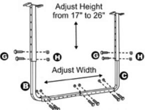
Assemble (2) Corner Rods (B & C) to each of the Support Bars (D & E) by sliding one inside the other as shown. Determine the length down from the ceiling you want the unit to hang (from 17" to 26").
