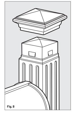
**STEP 8** Attach the Pyramid Finial to the top of the Upper Post Section by pressing and snapping firmly into place.
