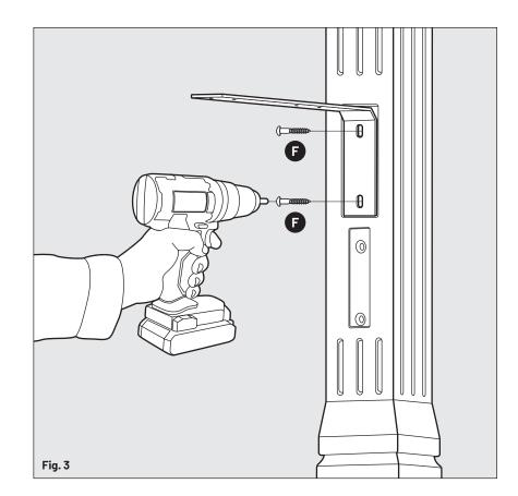
**STEP 3** Attach the Steel L Bracket to the Upper Post Component using the (2) #14 x 1-1/2" Pan Head Screws (3) included in the kit.
