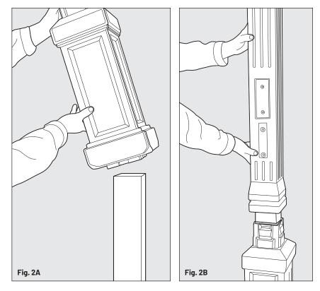
**STEP 2** Slide the Lower Post Section over the wooden post. **NOTE:** there is not a "front" to this section, so it does not matter what side is facing the street. Secondly, slide the Upper Post Section over the wooden post. **NOTE:** make sure the side with the part / screw pattern (shown in Fig. 2B) is facing the street. Press the Upper Section onto the Lower Section until the two components snap together completely.
