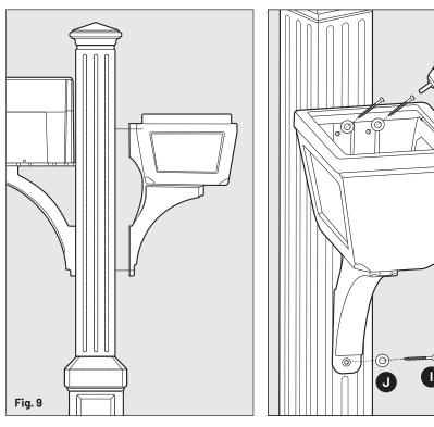
**STEP 9** Attach the Planter to the post. Locate the small dimple impression on the rear of the post section. Line up the hole at the bottom of the support brace with the dimple impression and secure using (1) 2" Wood Screw **①** and (1) washer **①**. Make sure that planter is centered with the post – then finish securing the planter to the post using the 2 remaining wood screws and washers as shown in the diagram above.
