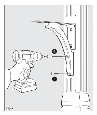
**STEP 4** Attach the Decorative Support Piece to the Upper Post Component using (1) #14 x 3" Pan Head Screw ③ in the upper hole and using (1) #14 x 1-1/2" Pan Head Screw ④ in the lower hole. Both of these screws are included in the kit.
