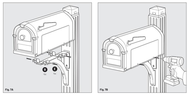
STEP 7 Securely attach your mailbox to the Mounting Brackets using the (4) #10 – 24 x 1–1/2" Phillips Machine Bolts 🕑 and (4) #10 – 24 Nuts 🕄 (included in the hardware kit). (4) spacers are also included in the kit for mailboxes larger than 8" in width.
