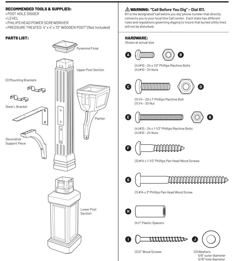
\*Actual Diameter of a Standard 4" x 4" Pressure Treated Post: 3-1/2" x 3-1/2" **PLEASE NOTE:** Concrete may be needed if installing in loose soil
