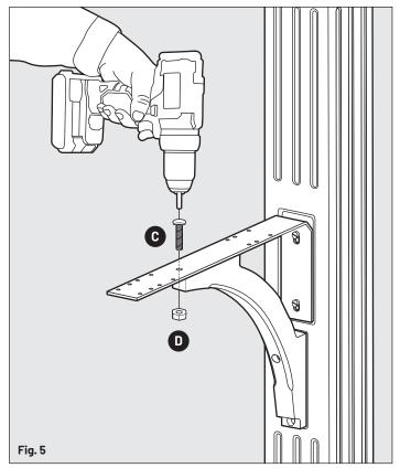
**STEP 5** Connect the Decorative Support Piece to the Steel L Bracket using (1)  $1/4 - 20 \times 1^{\circ}$  Phillips Machine Bolt (and (1)  $1/4^{\circ} - 20$  Nut (). This bolt and nut are included in the kit.
