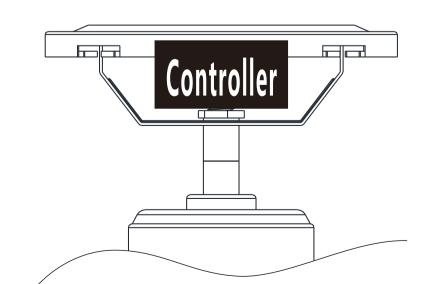
1:Remove the mounting bracket from the canopy by loosening the two canopy screws located in the L shaped slots.2:Remove and save the two canopy screws in the round holes. This will enable you to remove the mountingbracket
