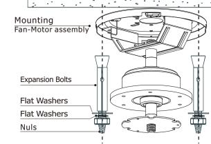
For concrete ceiling, use the percussion bit with diameter 8mm to drill holes according to the length of expansion screws. Then use the attached expansion screws to fix the hanging bracket onto the ceiling (selection is made according to actual requirements of the customers).
