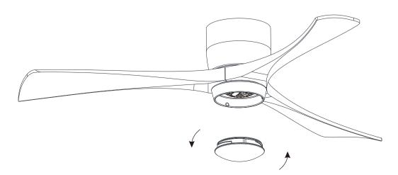
1. Screw the glass lampshade into the lamp in a counterclockwise direction. Make sure the glass lampshade is locked.
