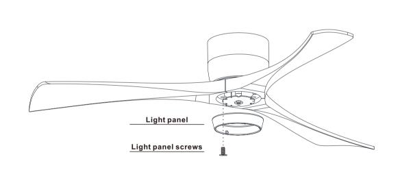
1.Remove the pre installed screws and install the lamp at the specified position
