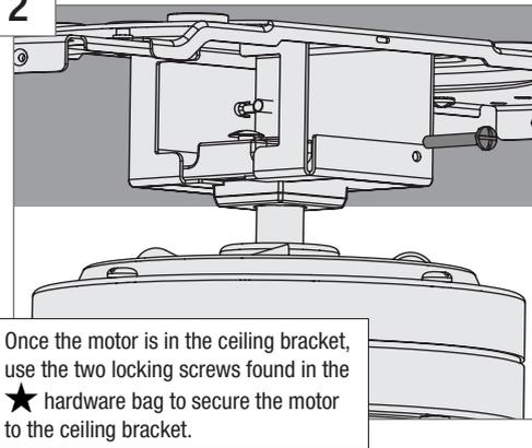
Once the motor is in the ceiling bracket, use the two locking screws found in the ★ hardware bag to secure the motor to the ceiling bracket.
