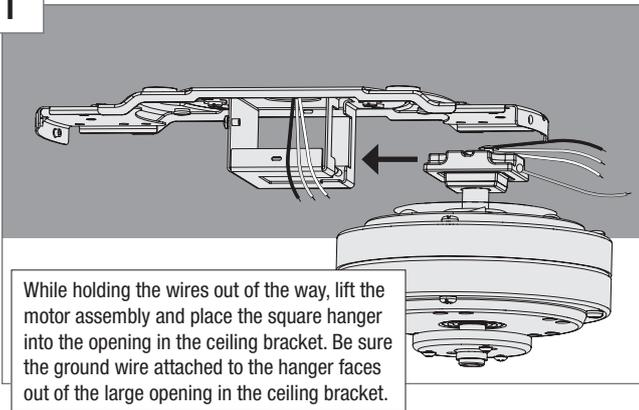
While holding the wires out of the way, lift the motor assembly and place the square hanger into the opening in the ceiling bracket. Be sure the ground wire attached to the hanger faces out of the large opening in the ceiling bracket.
