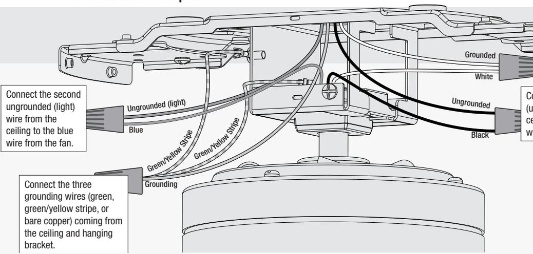
Connect the second ungrounded (light) wire from the ceiling to the blue wire from the fan.
