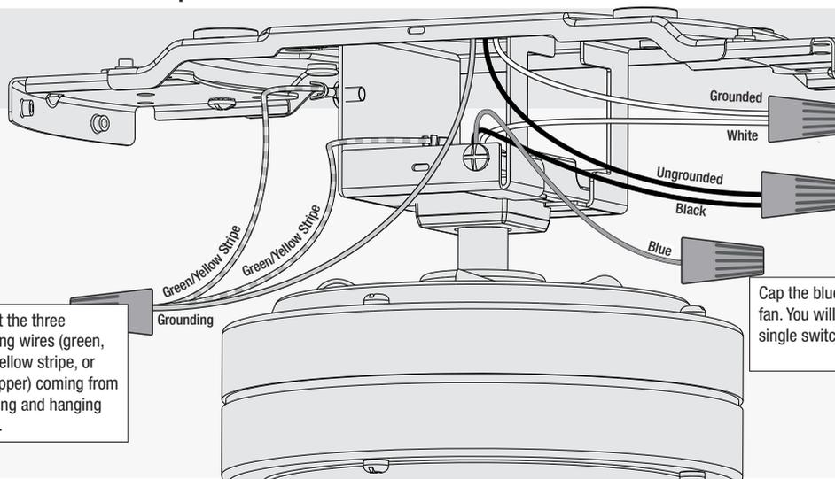
Connect the three grounding wires (green, green/yellow stripe, or bare copper) coming from the ceiling and hanging bracket.
