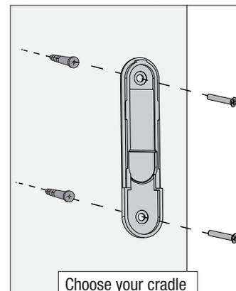
*If you are installing into drywall, drill two 9/64 width holes using the cradle bracket as a guide. Gently hammer the included drywall anchors into the pre-drilled holes.*
