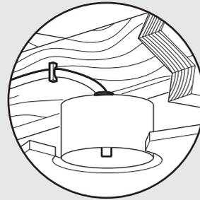
You must be able to secure the fan to building structure or fan-rated outlet box.
