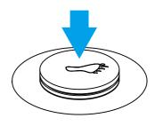
As the picture showed above, the drain is open. Step on it once, then close the drain; Step on it again, and then open the drain again.
