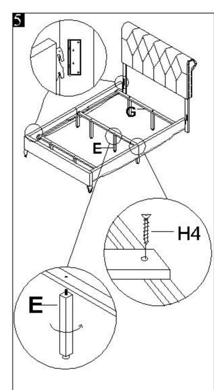
Attach 2 rails to the L/R posts & the footboard assembled with legs.
