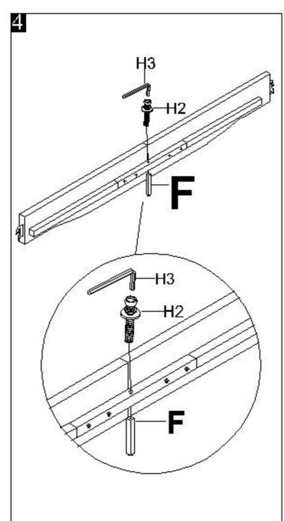
Attach support legs "F" to wood bar "L" .Using wrench (H3) to lock with bolts "H2".
