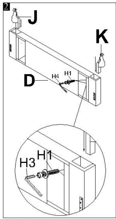
Attach wood legs "J" & " K" with footboard "D". Using wrench (H3) to lock with bolts "H1".
