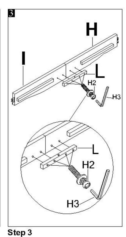
Attach wood bar "L" to the 2 rails "H" & "I". Using wrench (H3) to lock with bolts "H2".
