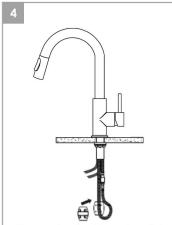
Connect pullout hose to quick connect and insert weight (looseinstall)
