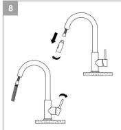
Unscrew spray head by hand. Hold the tip of the spray hose down and turn on the faucet and let the water run 60 seconds to flush any debris, the re-connect spray head. Ensure gasket is present.
