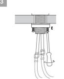
Position faucet on the installation surface. Fit flexible hoses through hole on countertop or sink.
