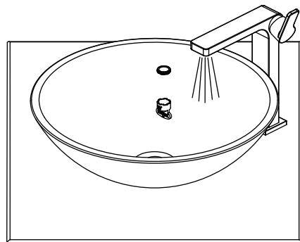
**Note:** Screen washers have been added to the supply lines. If flow becomes restricted or pressure reduced, please proceed as follows: Shut off water supply at angle stop and unscrew the hoses from water supply lines. Remove screen washers (2) from hoses (1) and clean/rinse off any debris. Reinstall the washers (2) into hoses (1) in original direction, reconnect supply lines and turn water on.
