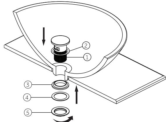
6. Slide the nut (2) over the tailpiece (3). Place the washer (1) into the nut and tighten. Do not overtighten.
