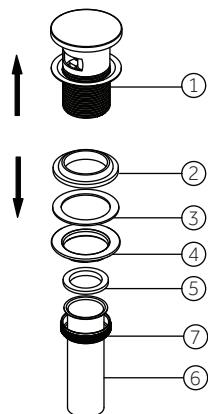
5. Place the washer (2) underneath the flange of the pop-up body (1). Slide the pop-up body (1) down through the drain hole on the vessel or basin. From underside of the sink, slide the beveled washer (3 & 4) against the bottom of the vessel or basin, thread on the coupling nut (5) and tighten. Do not overtighten.
