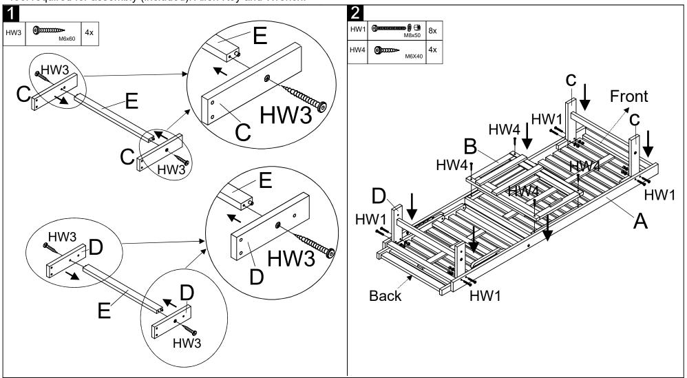
Step 1: Attach the Long leg (C) and Short leg (D) to the Support (E) as shown on the picture. Using the Screw L (HW3) and tighten with the Allen key (HW6) as shown on the picture.
