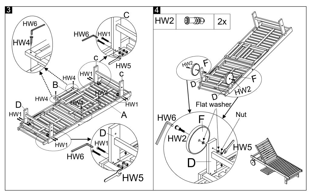
Step 3: Tighten all Bolt &nut (HW1) and Screw S (HW4) by using the Wrench (HW5) and Allen key (HW6) as shown on the picture.
