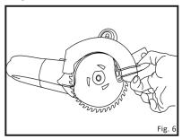
6. Lift up and remove "Face 2" blade. (Fig. 8)
