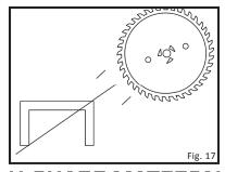
**U-SHAPE MATERIAL** Move blades to the U-profile material from the diagonal direction. (Fig. 17)
