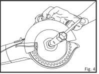
3. Remove lock nut and washer from the blade (fig. 5)
