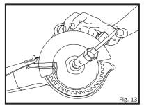
2. Open lower guard and place "Face 2" blade on saw and fit on the outer arbor shaft . (Fig. 10)
