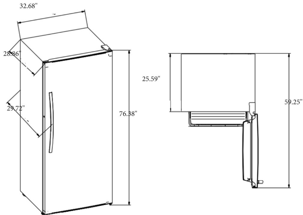
Keep enough clearance between the appliance and its surroundings to ensure the function of the appliance.
