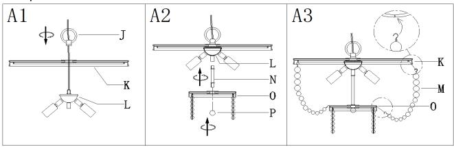
Step A1: Pass fixture loop assembly (L) through upper iron ring (K) and secure with loop (J).
