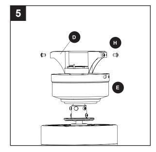
6. Attach mounting bracket (D) to outlet box (not included) using screws and washers provided with the outlet box.
