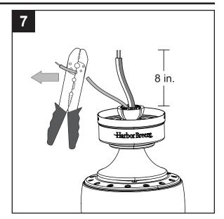
8. If you decided to cut back the lead wire in Step 7, strip 1/2 in. of insulation from the end of the white wire. Twist the stripped ends of each strand of wire within the insulation with pliers (not included). Repeat this step for black and blue wires.
