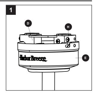
2. Secure the canopy (E) with the mounting bracket screws (H) previously removed (Step 5, page 8). Tighten all mounting bracket screws (H) securely.
