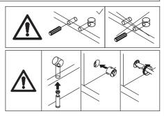
Attach board 13 to board 7, add cam lock(B) into board 13 and turn clockwise to tighten as shown.
