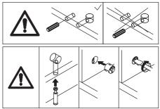
Connect assembled components, add cam lock(B) into and turn clockwise to tighten as shown. Insert wooden dowel(D) into board 15 as shown.
