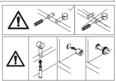
Connect the two assembled components, add cam lock(B) into and turn clockwise to tighten as shown.
