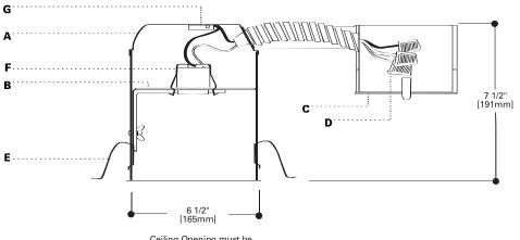
Ceiling Opening must be cut to match template supplied with housing
