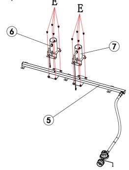
Assemble the burner-short line (6) and the burner-long line (7) to the burner bracket (5) with 8 bolts (E) as shown.
