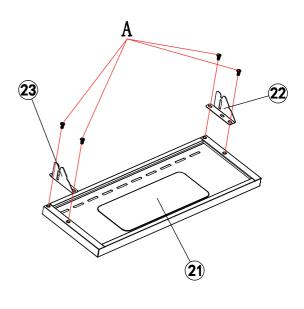
Install the bracket - left (22) and bracket - right (23) to the front table (21) with 4 bolts (A).
