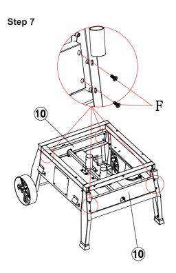
Assemble the side panel (10) to the cart with 8 bolts (F) as shown.
