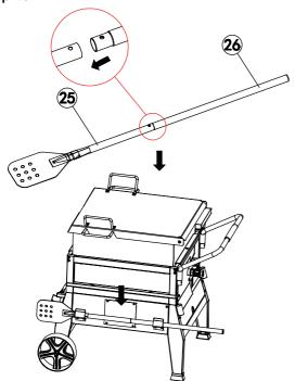
Press the spring and then put paddle (25) and hand lever (26) together.
