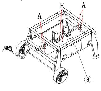
Install the burner bracket and base plate (8) to the cart with 4 bolts (A) and 2 bolts (E) as shown.
