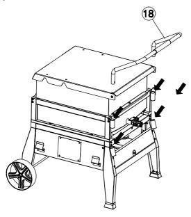
Insert the side handle (18) to upper position for transportation, and lower position for dumping.
