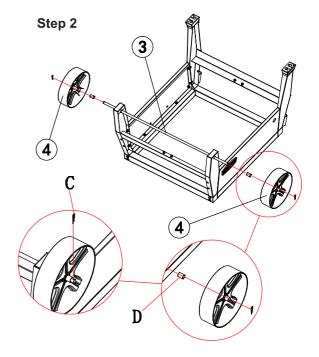
Slide the wheel axle (3) through legs. Slide the spacers (D) prior to install the steel wheels (4). Secure wheels by inserting the split pins (C) on axle.
