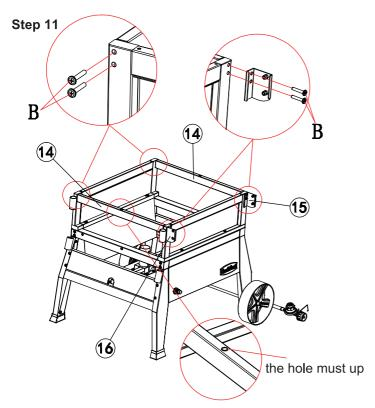
Assemble the tube support - boilers (14) and the front table joints (15,16) to the cart with 8 bolts (B) as shown.
