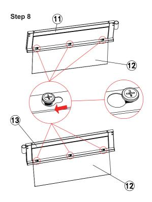
Loose the 6 preassembly bolts on the front panel - boiler (11) and back panel - boiler (13), then attach the thermal baffle (12) as shown.
