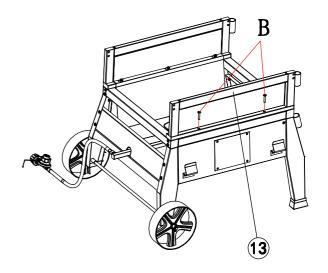
Install the front panel - boiler (11) to the cart with 2 bolts (B).
