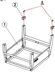
Install the feet (2) to the left legs with 4 bolts (A).
