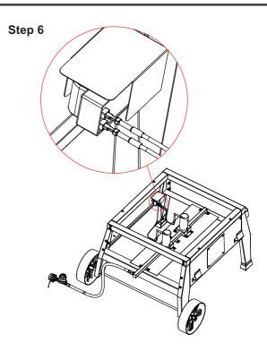
Insert the electrode wires to ignitor.
