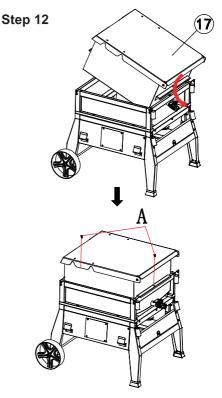
Put the drain valve in as indicated, then install the boiler body (17) into the cart with 2 bolts (A) .
