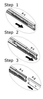
Before installation, slide the inner iron pieces of #F-1 to the outermost side.
