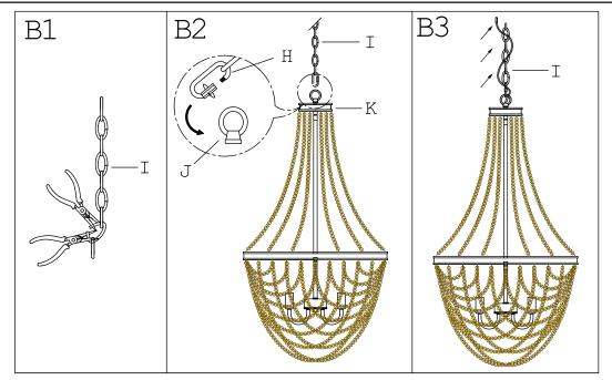
Step B1 » By measuring, determine the correct number of links needed for proper hanging height. Using the chain pliers, disconnect and discard the unwanted part.
