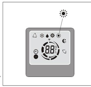
• During heating mode, the unit can automatically activate a defrost cycle, which is essential to clear the condenser from a excess desposit of frost. The process usually lasts for 2-10 minutes and during defrosting, the fan will stop operating. After completing the defrost cycle, it will return to heating mode automatically.
