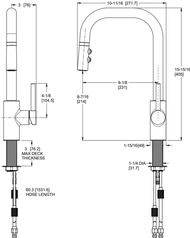
Ø1-3/8 Min to Ø1-1/2 Max. Deck Hole Openings
