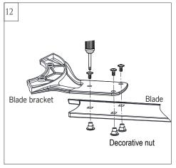
Install blade bracket with blade by 3 blade screws and decorative nuts provided. Tighten screws securely. Repeat this process for remaining blades.
