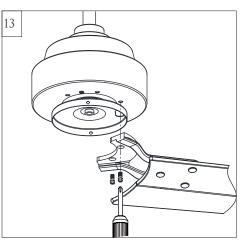
Install the blade assembly to motor using the set screws provided. Tighten screws securely. Repeat this process for remaining blade assemblies.
