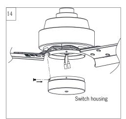
Remove set screws from switch housing. Keep screws.
