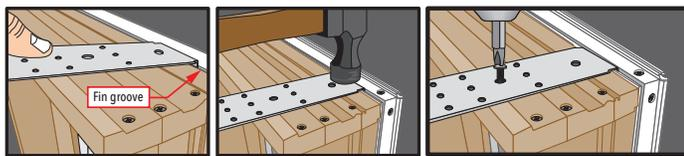
Alternatively, it is acceptable to use two #6 x 5/8" screws through the clip with the clip on its back and not engaged in the fin groove.
