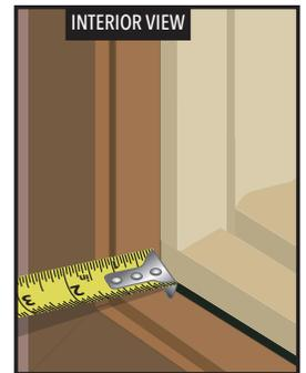
**NOTE: Keep shims 1/2" from the interior surface of the window to allow for a continuous interior seal and 1/2" from the exterior surface of the window to allow for exterior backer rod and sealant.**
