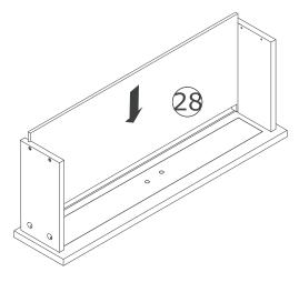
Insert bottom board 28 along available grooves as shown.
