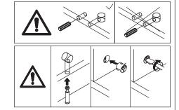
Connect board 8 to board 16 using LONG wooden dowel(G), and fix with screw(D) as shown.
